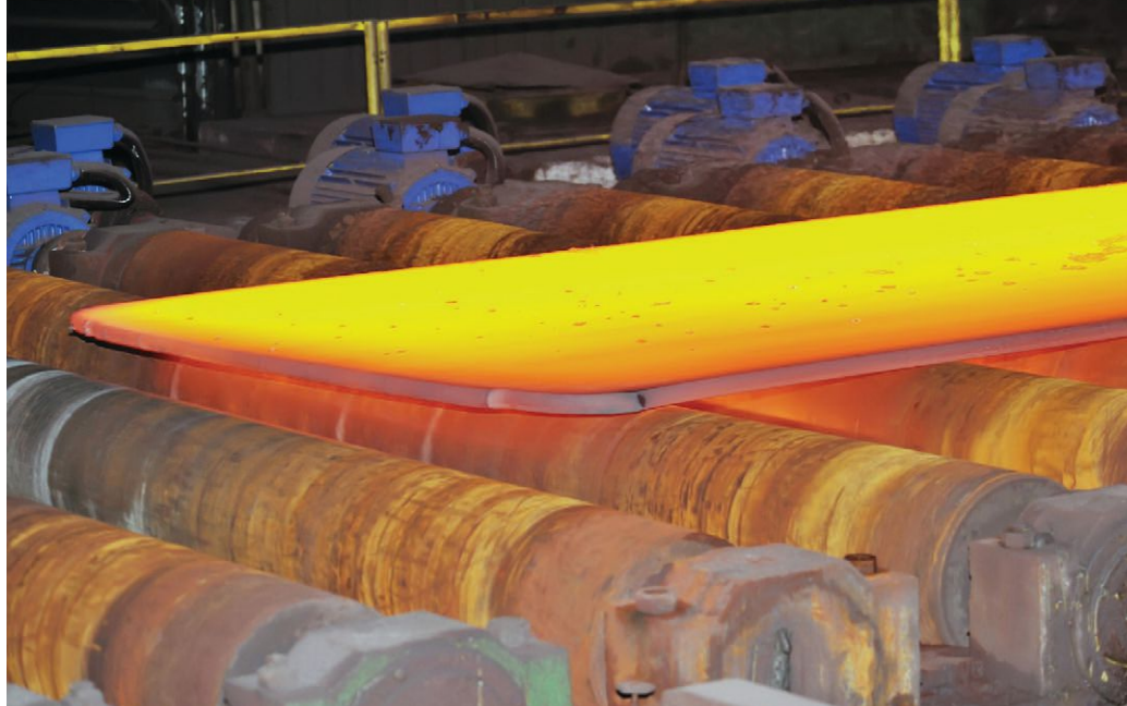
High temperatures and heavy shear are typical in steel mills. Frequently, high loads require potent extreme pressure additives.
